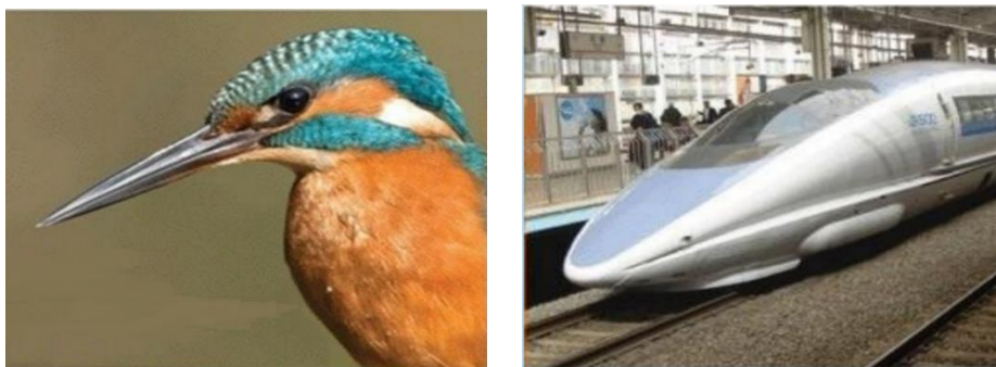
Figure 1. Kingfisher's beak inspired the Shinkansen trains' nose section design.
